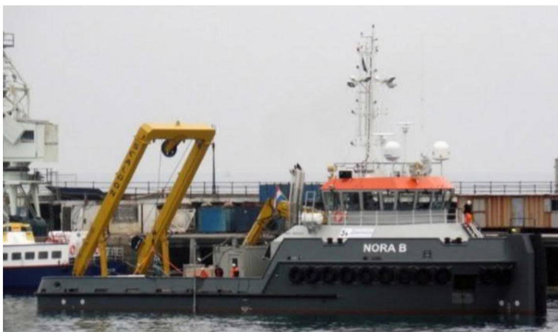
Figure 2.22: Example of a Pre-Lay Grapnel launch vessel
