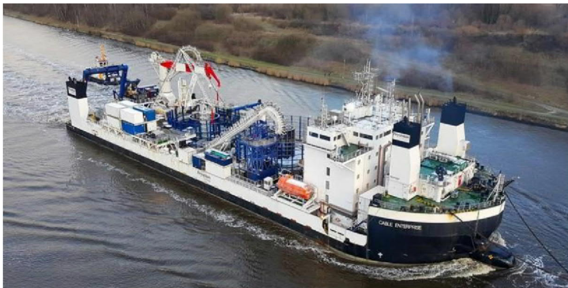
Figure 2.20: Example of a primary Cable Laying Barge [approximate size 125m (l) x 32m (b)]
