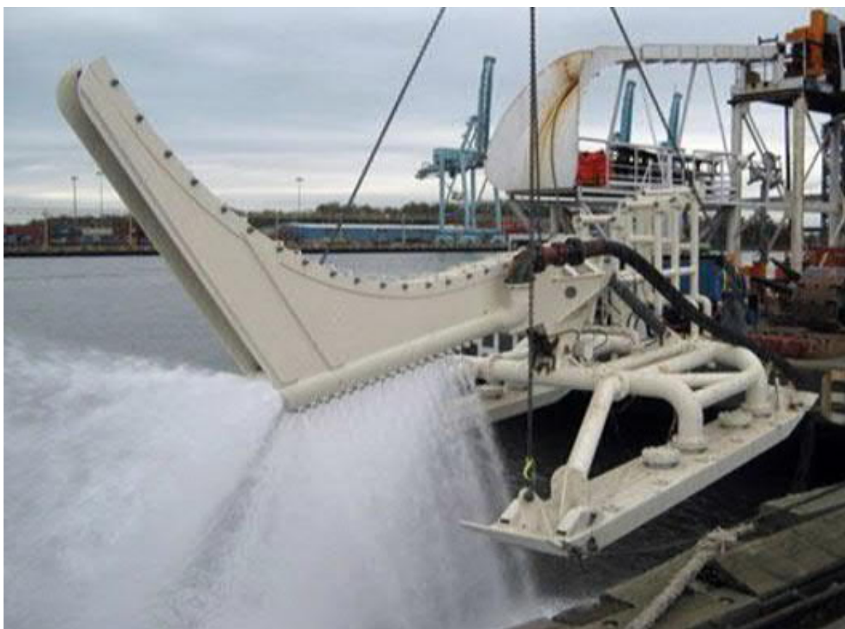
Figure 2.24: An example of a jetting tool
