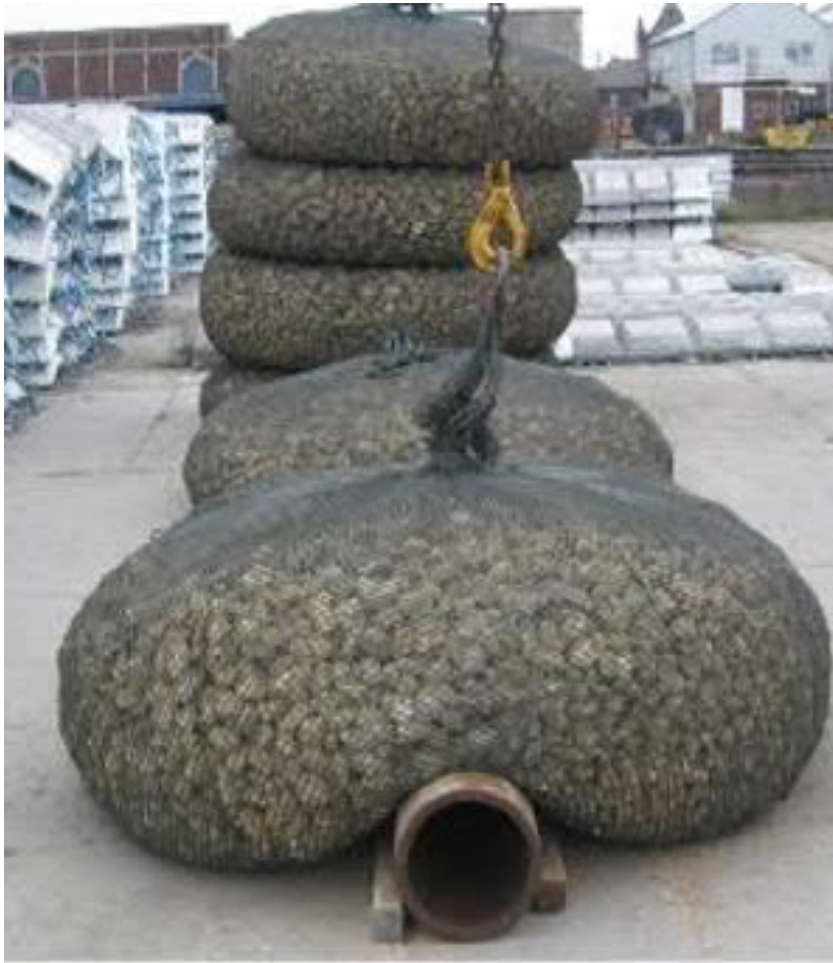
Figure 2.15: Example of Cable Protection Rock Filter Bags
