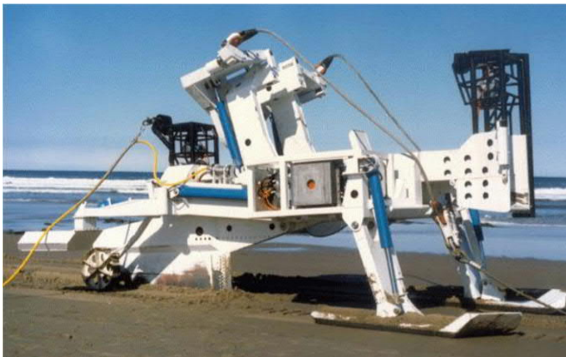
Figure 2.21: Example of a cable plough tool
